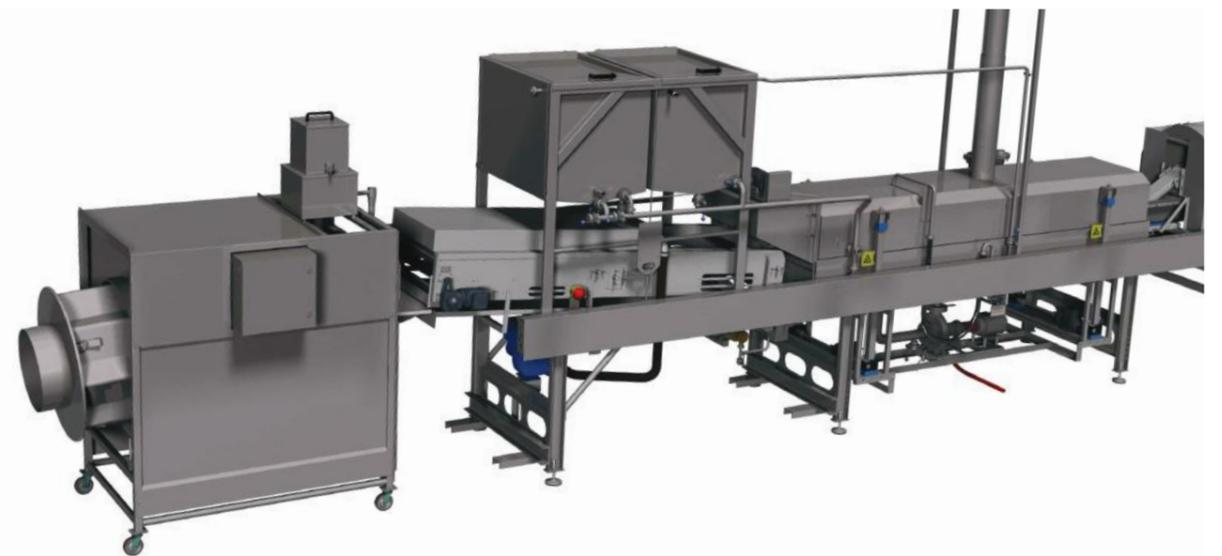
Deep frying depends largely on maintaining oil of the best quality. Thanks to the specially developed dirt removal system, combined with gentle heat treatment the oil does not have to be replaced - and without the addition of any chemicals. In fact, efficient removal of small particles begins before frying to prevent these from entering the frying system. This is another factor that contributes to an extremely low frying oil turnover time, in most cases less than three hours.
